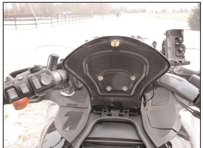
View of inside lid with 4 bolts that holds the Corona Mount in place
