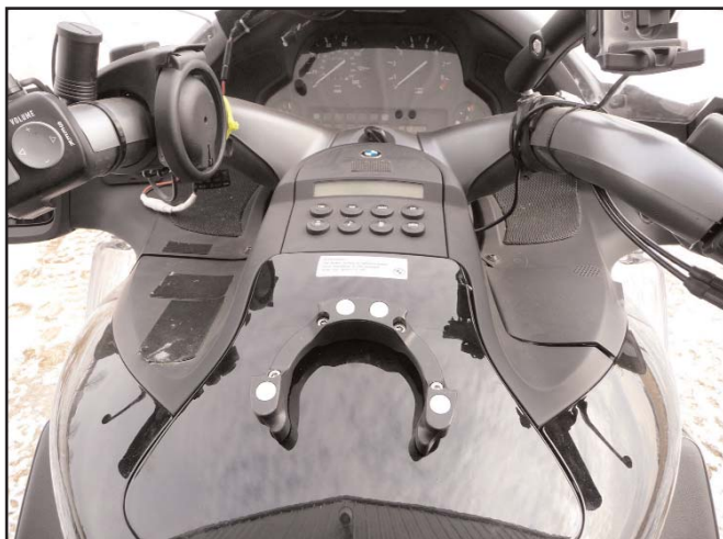
View of top of oddments box lid with Corona Mount in place
